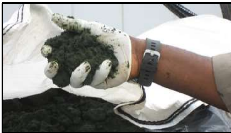
Picture 2: Crude cobalt hydroxide exported from the DRC (Picture taken by Marubeni's Johannesburg Branch expatriate staff.)
