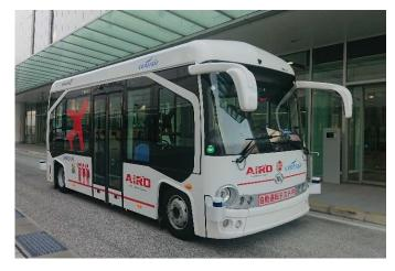
(\*) The autonomous driving Bus manufactured by ZMP, "RoboCar® Mini EV Bus"
