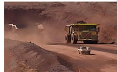
Large dump truck used to carry iron ore and dirt (Roy Hill Iron Ore Project, Australia)
