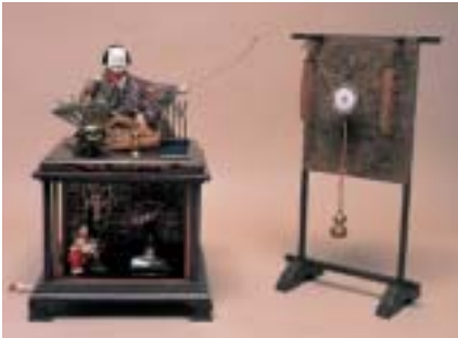
Karakuri (mechanical) puppet of a child with bow and arrow originally created by Hisashige Tanaka. The puppet shoots arrows at the target.
