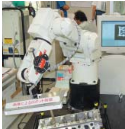
This robot compensates for object inclination and corrects its path using image-based technology
