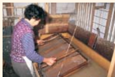
Fibers are entwined by shaking the tray side to side, and up and down when making paper
